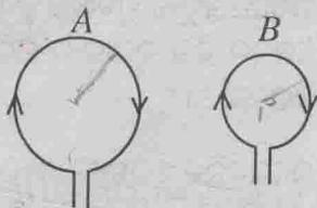
A and B are two circular conductors of the same material and thickness carry the same amount of current. The number of turns in 'B' is twice that of A, but radius of 'B' half of that of A. The ratio of the strength of the magnetic field at the center of 'B' and that of 'A' is
